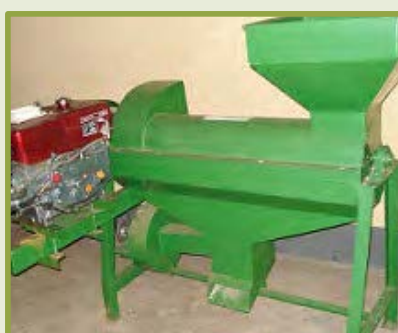
Locally fabricated non mobile motorised maize sheller
