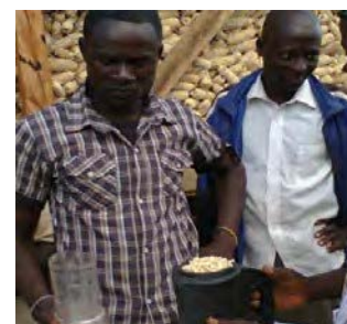
Testing MC using a moisture meter
